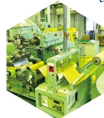
Extrusion Laminating Equipment
